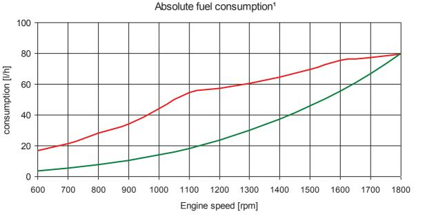
full load curve ----- propeller curve
