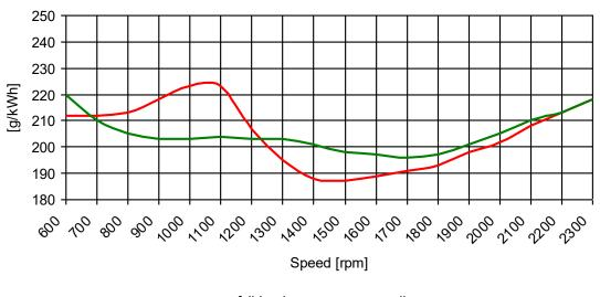
full load curve —— propeller curve
